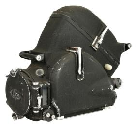
327.Ω **An Arri Arriflex Blimp,** 1960-, for use with Arriflex 16 cameras
