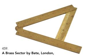
English, early 19th Century, signed in script 'Bate, London, with hinged strut, finely engraved with a full set of scales in the English pattern, engraved with trigonometrical and navigational scales, the addition of sundial-making scales to reverse, outer edge with 12" scale
